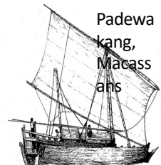
Illustration 1: A Padewa, a traditional Makassar sailing boat. This was the type of padewa most commonly used by the Makassar.
