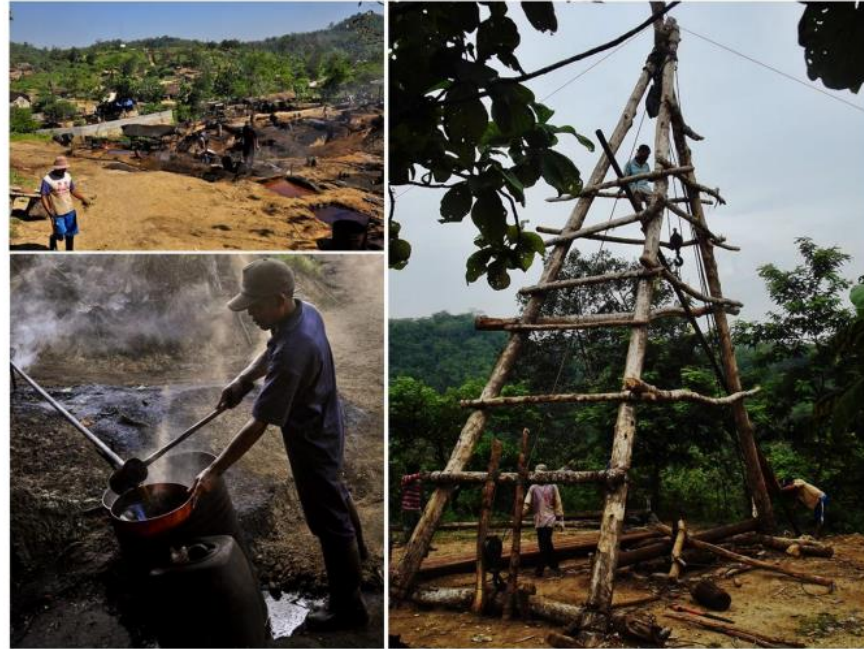
Figure 9. (upper left) scenery of traditional oil mining in Wonocolo Village (photo : Alan Yudhis); (lower left) final residue of traditional distillation. One well could produce 2-3 barrel oil of diesel and gasoline; (right) wooden oil rig.
