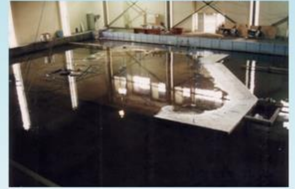
The 3-dimensional wave basin arrangement at Coastal Engineering Laboratory BPPT Yogyakarta (Now BDPD) for this undistorted model experiment (Prasetya, 1998)
