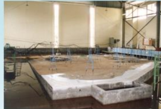
The 3-dimensional wave basin arrangement at Coastal Engineering Laboratory BPPT Yogyakarta (Now BDPD) for this undistorted model experiment (Prasetya, 1998)
