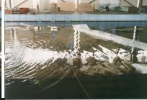
The 3-dimensional wave basin arrangement at Coastal Engineering Laboratory BPPT Yogyakarta (Now BDPD) for this undistorted model experiment (Prasetya, 1998)
