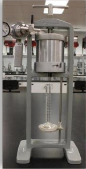
Filterpresses used for WBF testing
