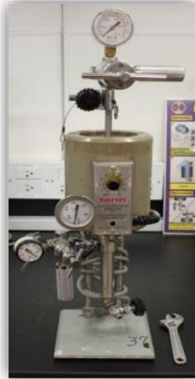
Filterpresses used for WBF testing
