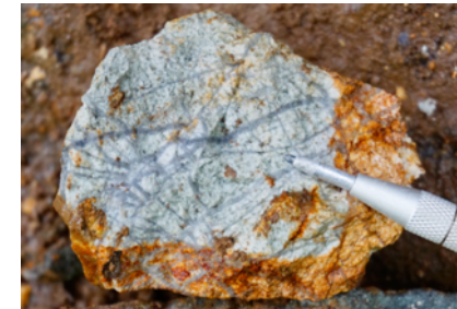
Quartz stockwork hosted by quartz-sericite altered Quartz Diorite in Anomaly 2 (0.67 ppm Au and 0.2% Cu)
