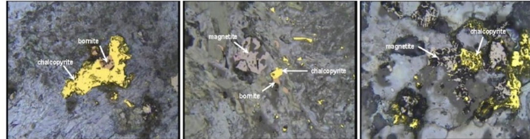
Disseminated chalcopyrite (yellow), bornite (purple grey) & magnetite (light grey) propylitic-potassic altered diorite (TRDD055 & 58)
